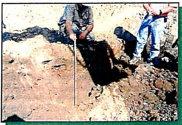
Figure 3-7: Using a backhoe, small trenches are dug perpendicular to the centerline of the historic ditch/canal. Samples are collected from the side walls and floor of the trench at 2-foot intervals (or on a 2-foot grid) or where the characteristics or strata of the soil change.
