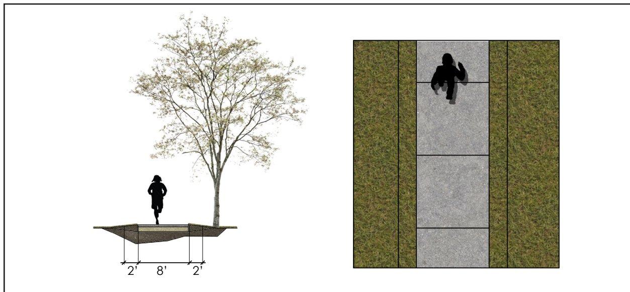
Figure 43: Typical cross section (left) and plan view (right) of an improved pedestrian trail.
