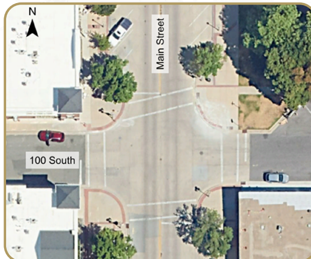
Example of intersection bulb out and on-street parking (aerial view) - Bountiful, UT
